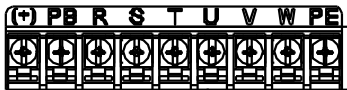
Figure 3-5 3PH terminals of main circuit (220V, \leq 0.75\text{kW} , and 380V, \leq 2.2\text{kW} )
